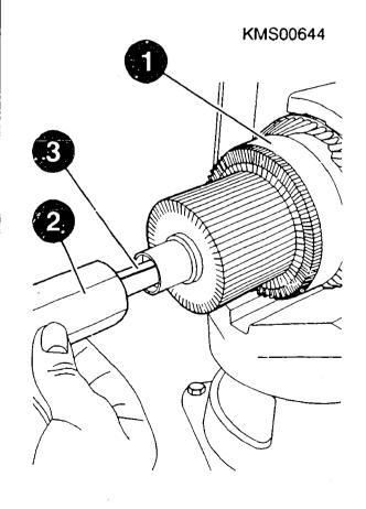
Replacing bushing in armature Installing:
